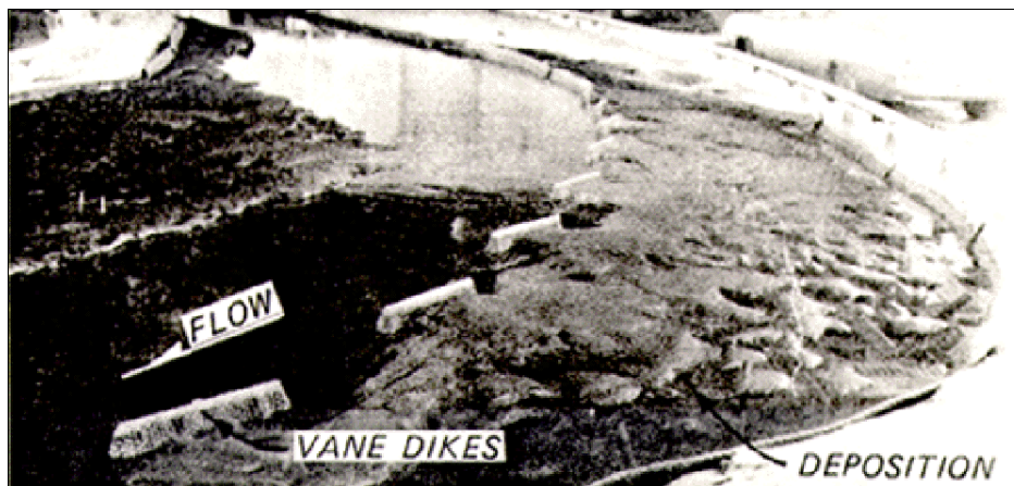
Figure 6.7. Vane dike model, ground walnut shell bed, during low stage portion of test run (U.S. Army Corps of Engineers 1981).
