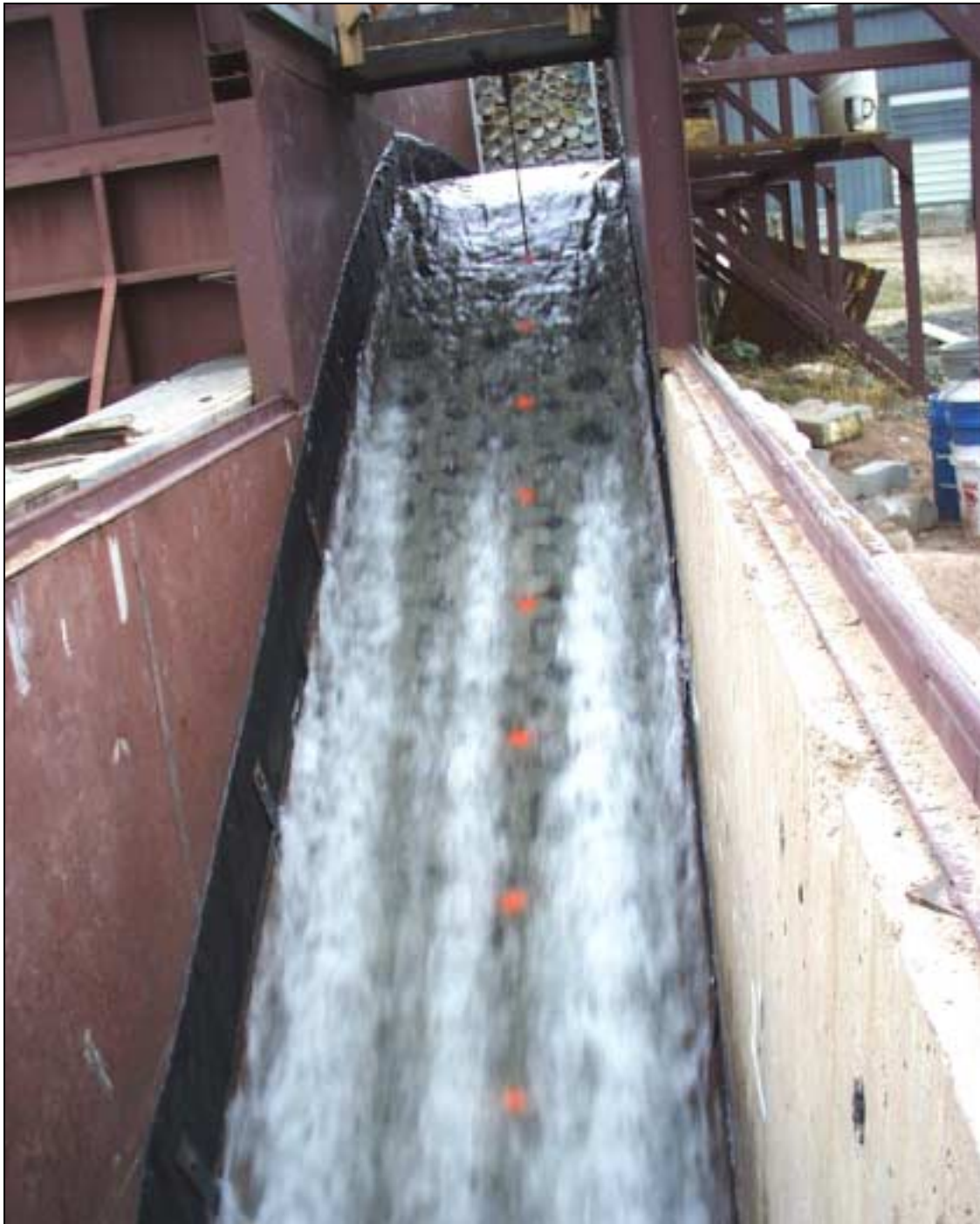
Figure 6.31. Full-scale test of an embankment overtopping protection system under steep-slope, high-velocity flow conditions.
